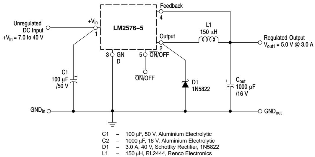
Figure 35. Schematic Diagram of the LM2576-5 Step-Down Converter
