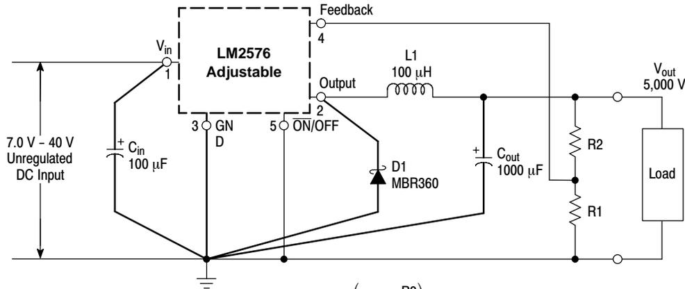
$$V_{out} = V_{ref} \left( 1.0 + \frac{R2}{R1} \right)$$
