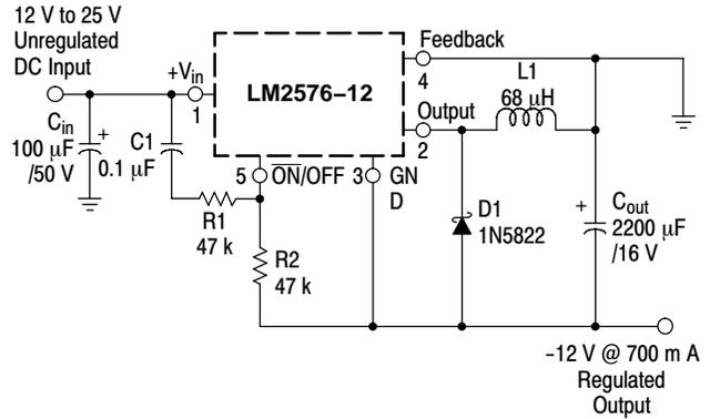
**Figure 27. Inverting Buck–Boost Regulator with Delayed startup**
