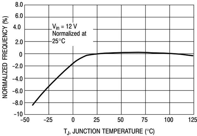
Figure 10. Oscillator Frequency
