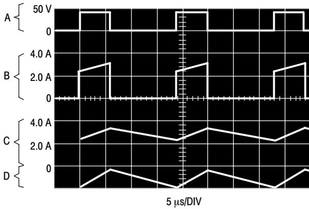
Figure 13. Switching Waveforms
